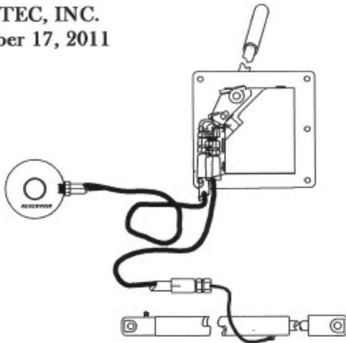
This unit is shipped primed with a reservoir hose plug, system pressure cap plug, and release valve closed.
